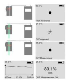
Freehand light transmission measurement: 1) 100% adjustment 2) sample alignment (DUT) 3) automatic measurement start upon setup, 4) Display of the measurement values
